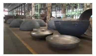
A tank dish end, also known as a tank head or tank cap, is a component used to close or seal the ends of cylindrical pressure vessels such as tanks, boilers, and reactors. These ends are curved in shape, resembling a portion of a sphere or ellipsoid, and are welded or bolted to the cylindrical body of the vessel. Tank dish ends serve several important functions in pressure vessel design and operation:
